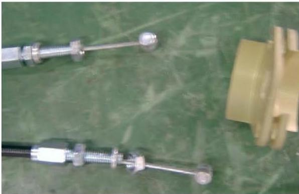
图 9 将拉线组件从联锁凸轮上取下
