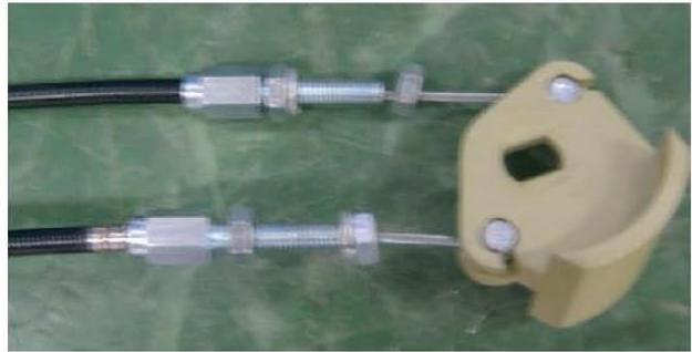
图 8 将拉线组件和凸轮一起从联锁支板上取下
